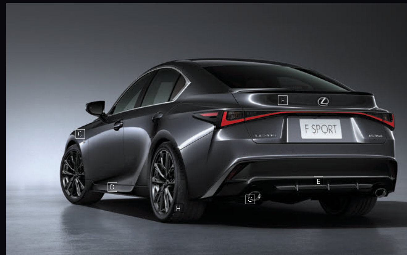
C_Front fender emblems / D_Side rocker moldings / E_Rear bumper / F_Rear spoiler / G_Mufflers / H_Aluminum wheels
