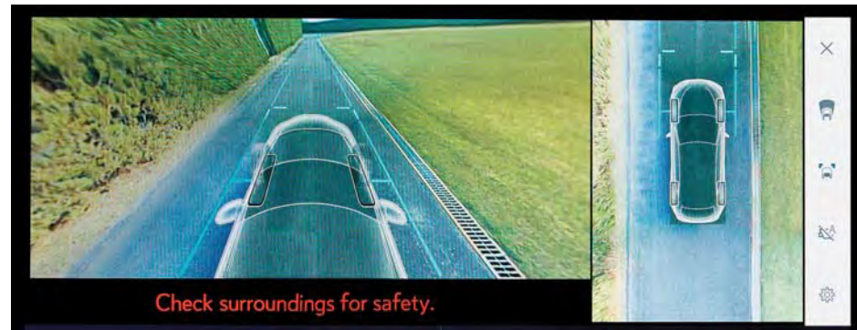
Panoramic View and Side Clearance View
